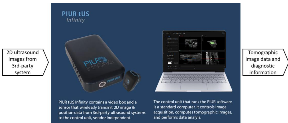
Figure 1: PIUR tUS Infinity system set-up
