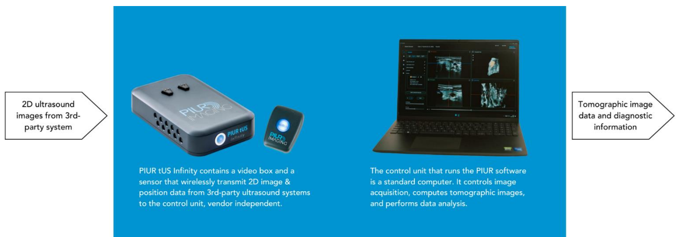
Figure 1: PIUR tUS Infinity system set-up
